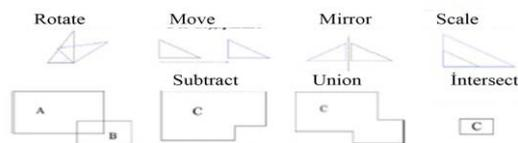
**Figure 2.** The formal transition codes used in shape Grammar [20].
