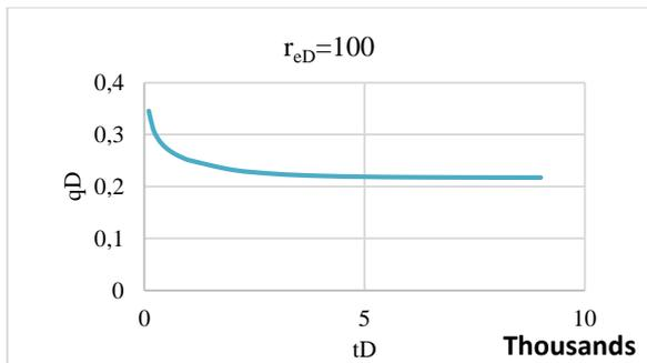
**Figure 2.** A graph of  $q_D$  against  $t_D$  at  $r_{eD}=100$
