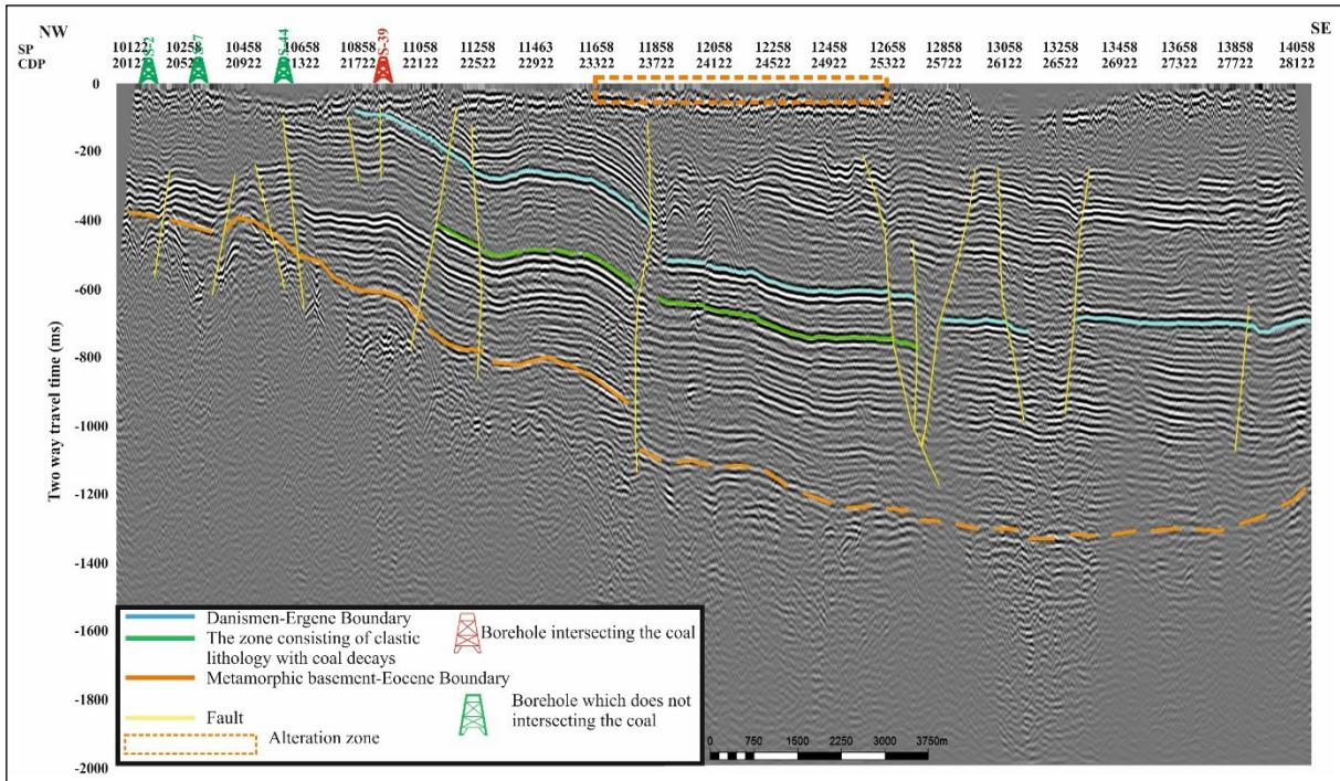
Figure 6- Interpreted KRKV1801 seismic cross-section. The small and large-scale faults that are not named and dominate throughout the region are shown in yellow. The location of the borehole intersecting the coal (S-39) is shown with a red symbol in the figure. The location of the boreholes which does not intersect the coal (S-2, S-7, and S-44) is shown with a green symbol in the figure. The boundary of the alteration zone is shown with the orange dashed line.
