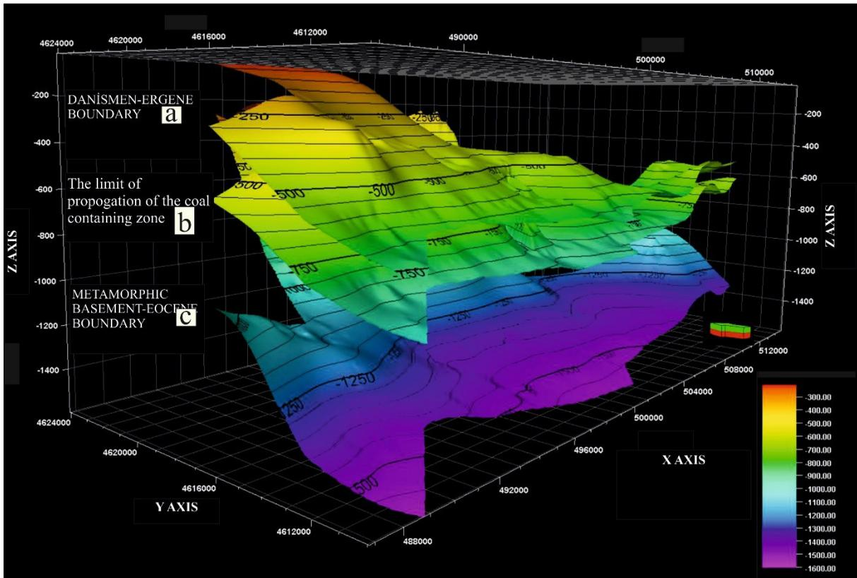
Figure 10- 3D view of; a) Danişmen-Ergene boundary, b) extensions of the coal-containing zone and c) metamorphic Basement-Eocene boundary. All boundaries are plotted on a millisecond (ms) scale.
