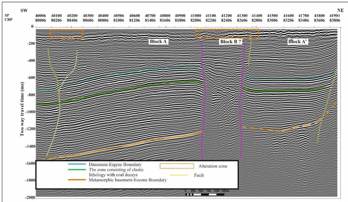
Figure 9- Interpreted KRKV1904 seismic cross-section. A possible strike-slip fault is shown in pink and the fault that is not named is shown in yellow. The boundary of the alteration zone is shown with the orange dashed line. It is seen that the seismic levels, which are colored blue, green, and orange, are followed along the line in blocks A and A' but in block B these seismic levels are deteriorating.
