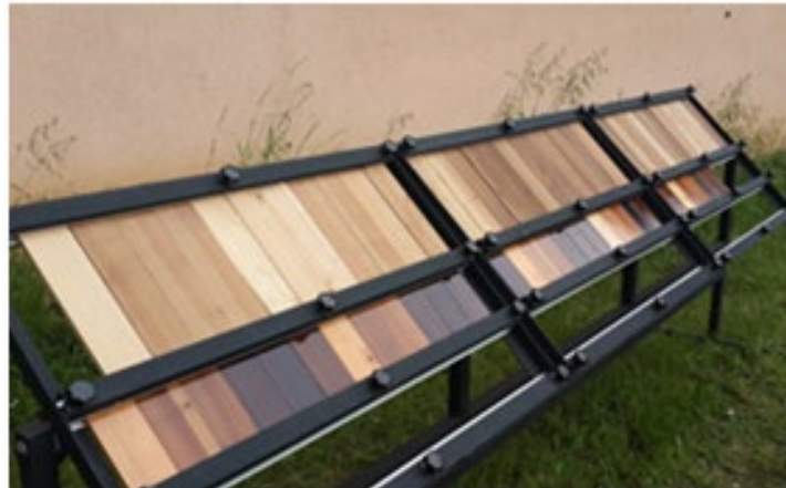
Figure 2: Natural weathering of test samples with an angle of 45°.
