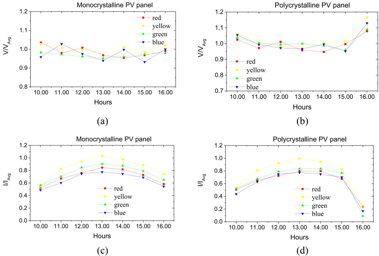
Fig. 5. Variation of voltage (a, b) and current (c, d) values of red, yellow, green, and blue filtered monocrystalline photovoltaic panel compared to the average voltage and current values of unfiltered monocrystalline and polycrystalline photovoltaic panel versus time
