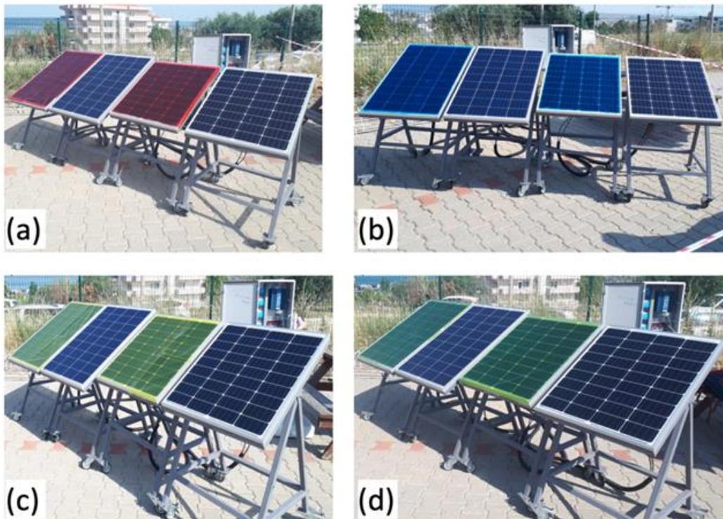
**Fig. 2.** Photovoltaic module without filter and with colored filters a) red, b) blue, c) yellow and d) green filters on the photovoltaic panels
