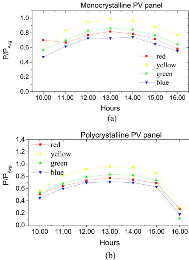
**Fig. 3.** Time variation of the power ratio of red, yellow, green, and blue filtered monocrystalline photovoltaic panel compared to the average power values of unfiltered monocrystalline (a) and polycrystalline (b) photovoltaic panels
