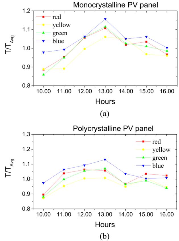
**Fig. 4.** Variation of temperature values of red, yellow, green, and blue filtered monocrystalline and polycrystalline photovoltaic panels compared to the average temperature values of unfiltered monocrystalline (a) and polycrystalline (b) photovoltaic panels versus time
