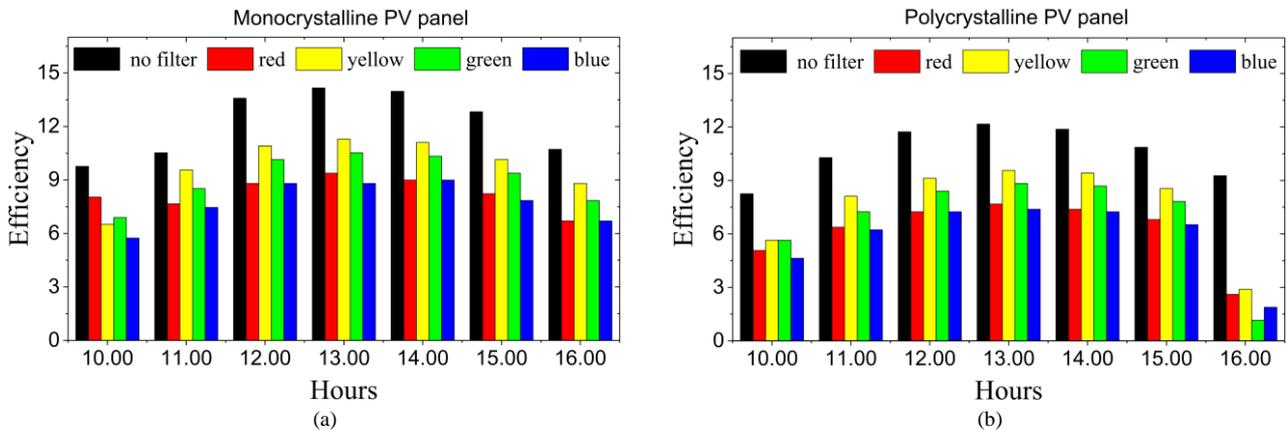
Fig. 6. Comparison of filtered and unfiltered monocrystalline (a) and polycrystalline (b) PV panel efficiencies over time
