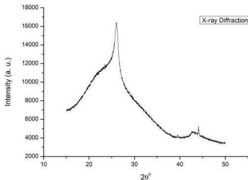
Figure 3 XRD analysis of Laser Scribed Graphene.
