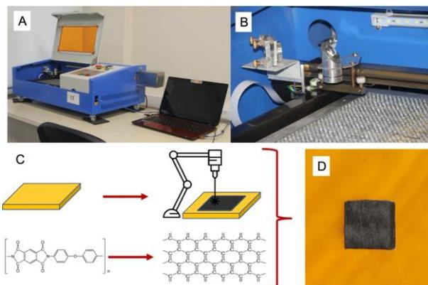
Figure 1 a) The K40 CO<sub>2</sub> laser system, b) Close up to optics, laser head, and sample stage c) Schematic representation of the working mechanism, d) Graphene film directly written on the PI surface.
