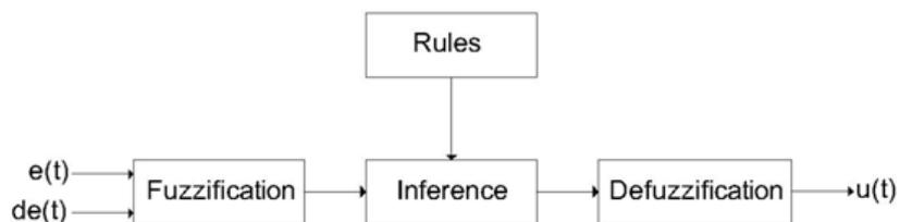
Figure3. General diagram of a fuzzy controller
