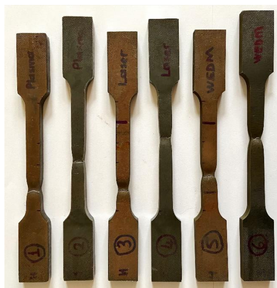
Fig 11. Fracture after tensile testing.
