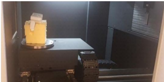
Figure 4. CT set-up consisting of the table and the part.
