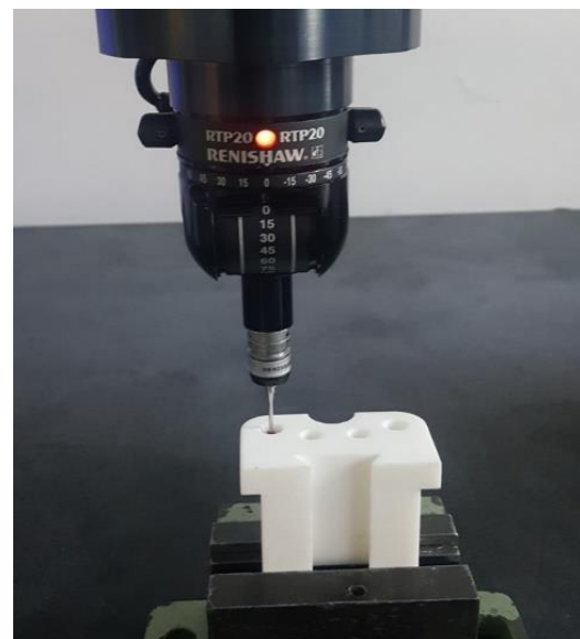
Figure 3. CMM set-up consisting of the vise and the part.
