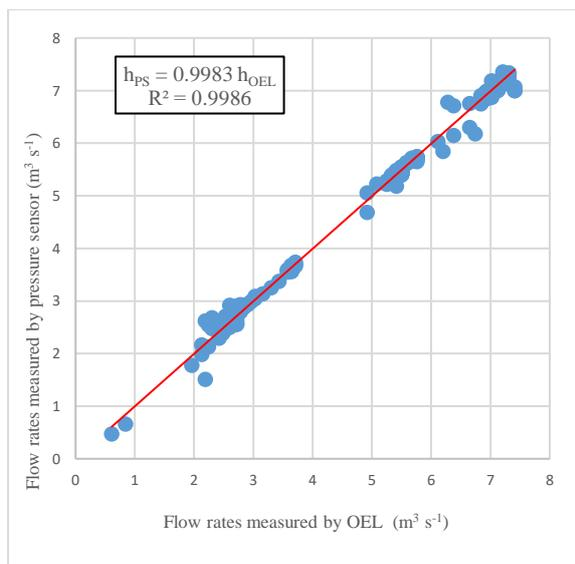
**Figure 5. Optic encoder limnigraph-pressure sensor flow rates**
