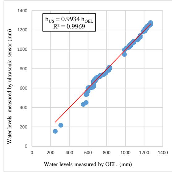
**Figure 4. Optic encoder limnigraph -ultrasonic sensor water levels**
