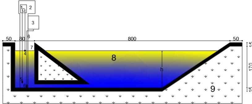
**Figure 1. Cross section of trapezoidal type main irrigation canal and FGS (1-Limnigraph, 2-Limnigraph shelter, 3-PLC panel, 4-Limnigraph ball, 5-Limnigraph weight, 6- pipe, 7-FGS box, 8- Water cross-section, 9 -Canal fill section)**
