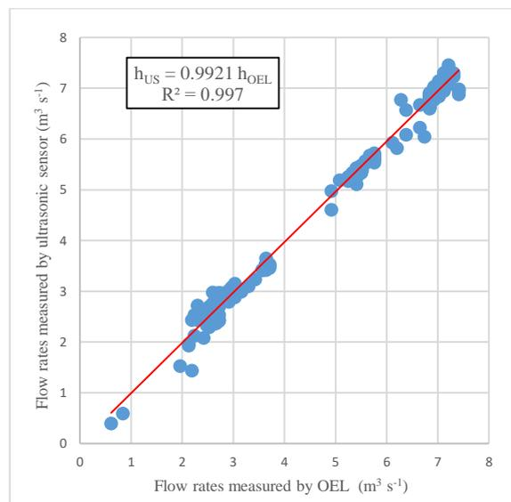
**Figure 6. Optic encoder limnigraph -ultrasonic sensor flow rates**
