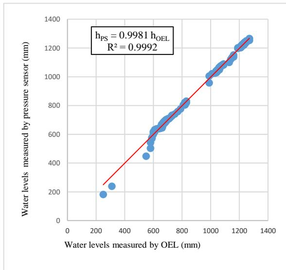
**Figure 3. Optic encoder limnigraph-pressure sensor water levels**
