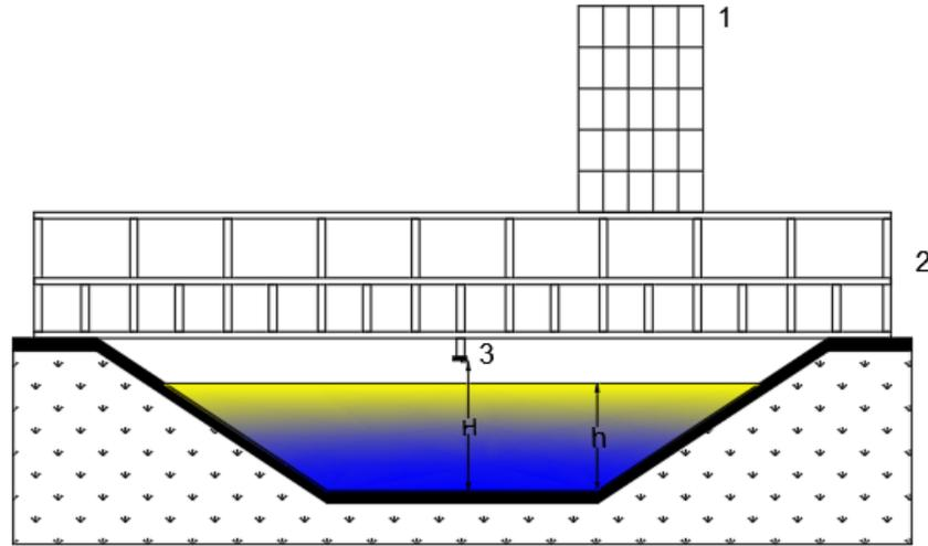
**Figure 2 Trapezoidal main canal, bridge section and solar panel (1-solar panel, 2-bridge, 3-ultrasonic sensor)**
