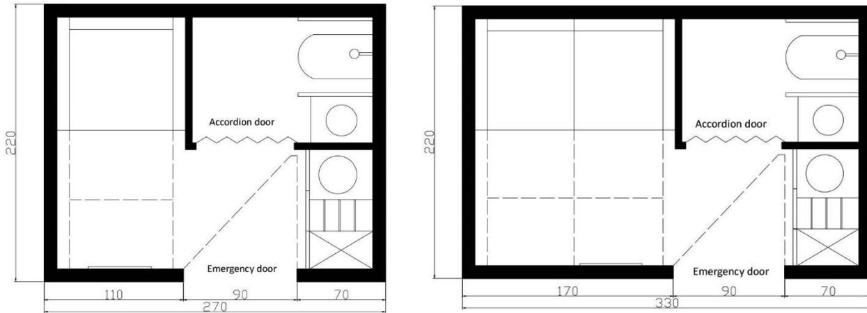
**Figure 1.** Plan for one user(Erten, ş. Y., AUTOCAD Software). **Figure 2.** Plan for two users (Erten, ş. Y., AUTOCAD Software).
