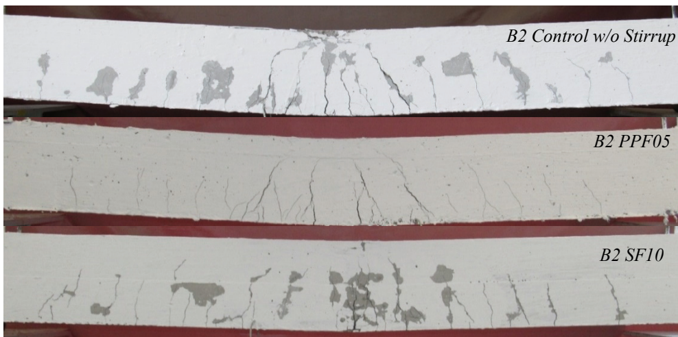
Figure 7 - Final state of crack patterns in B2 series
