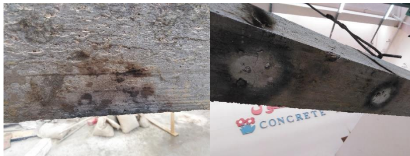
Figure 28. Surface changed color and charred
