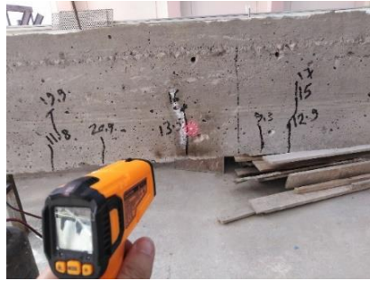
Figure 12. Recording the temperature at the evaluated points.
