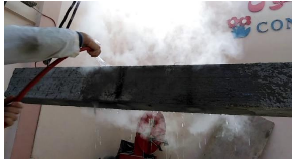
Figure 17. Cooling suddenly using the water
