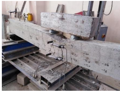
Figure 8. SCC beam fractured test.
