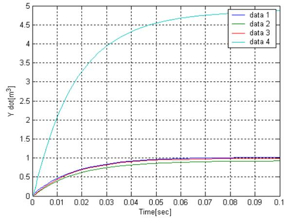
**Fig 1.3.** Effect of Restriction to flow on the Process, with  $R_1=0.1$
