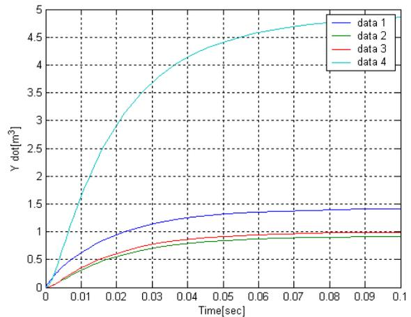
**Fig 1.5.** Effect of Restriction to flow on the Process, with  $R_1=0.5$
