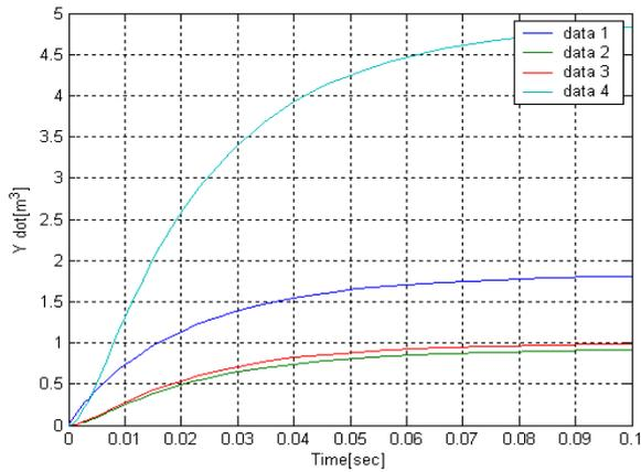
Fig 1.27. Effect of the Capacity of tank on the Process, with  $C_1 = 9e-03$
