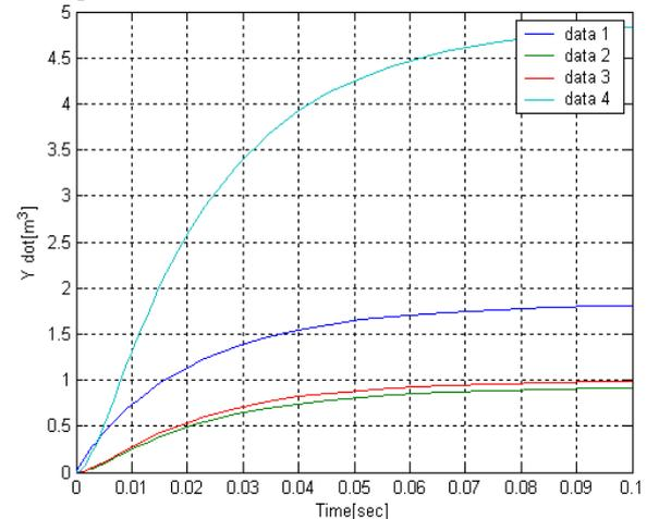
Fig 1.12. Effect of Restriction to flow on the Process, with  $R_2 = 0.9$
