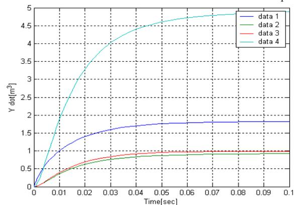
Fig 1.25. Effect of the Capacity of tank on the Process, with  $C_1=5e-03$
