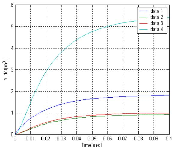
Fig 1.36. Effect of the Capacity of tank on the Process, with  $C_3 = 1700e-03$
