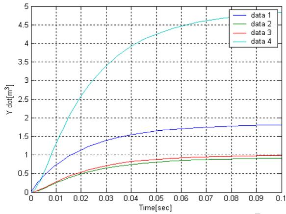
Fig 1.7. Effect of Restriction to flow on the Process, with  $R_1 = 0.9$
