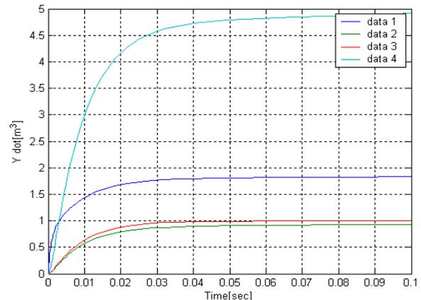
Fig 1.23. Effect of the Capacity of tank on the Process, with  $C_1=1e-03$
