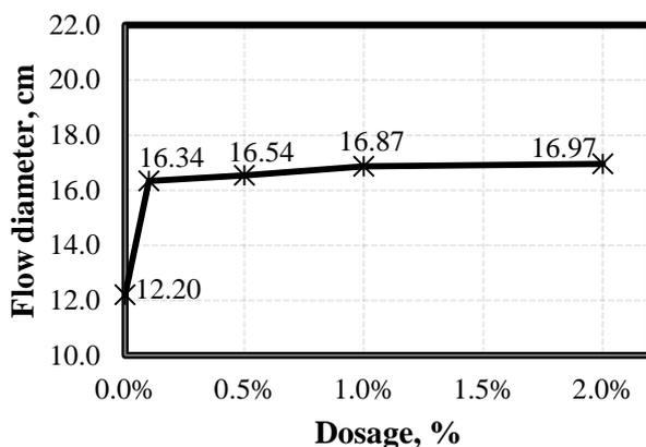
*Fig. 2. Flow diameter values obtained from flow table.*
