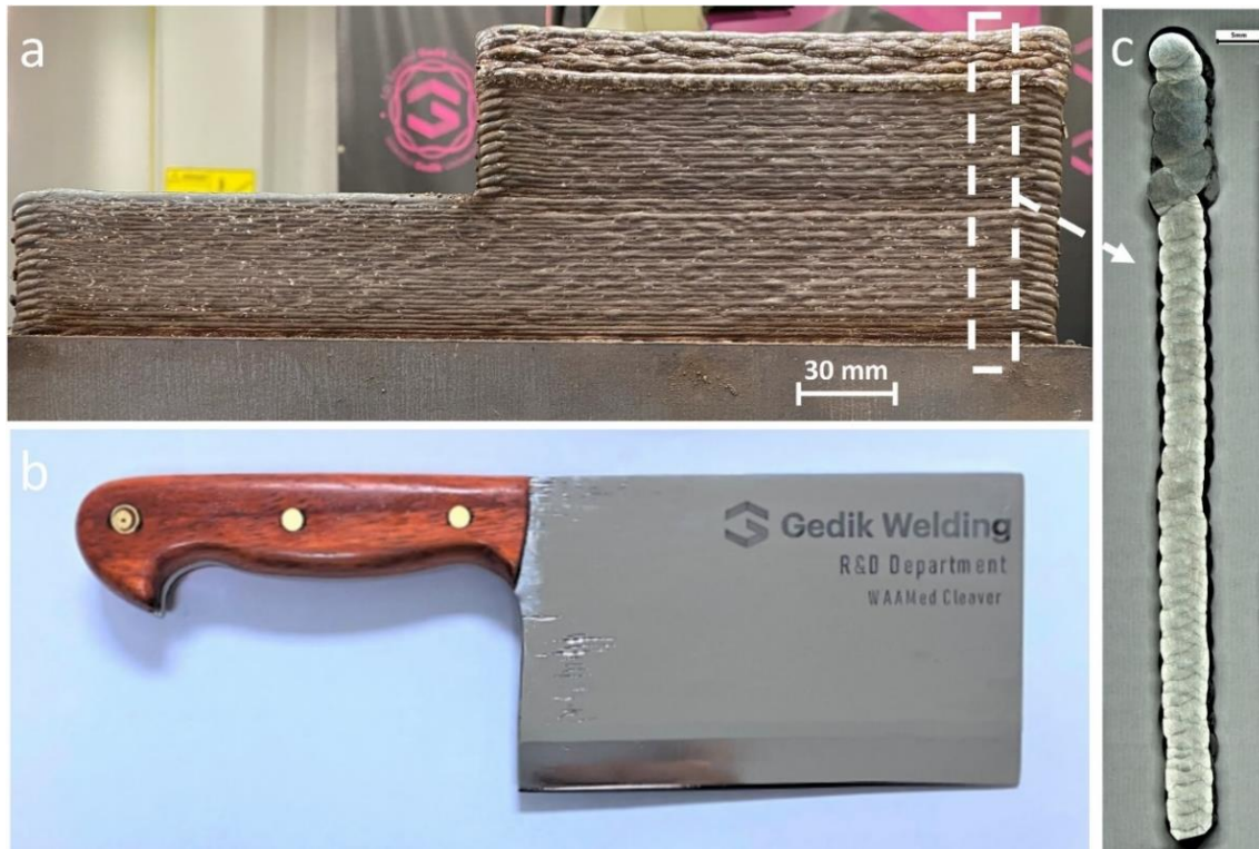
Figure 3. The general view of bi-material cleaver manufactured using WAAM technology and two different wires: a) as-printed, b) as-machined, c) macro structure of the cross-section of total 65 layers using two different wires.
