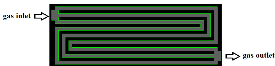
Figure 2. The bipolar plate flow channel pattern
