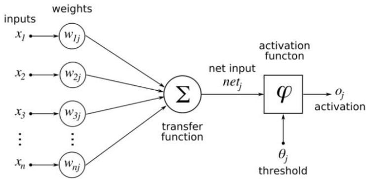
**Figure 2.** The working principle of the ANN
