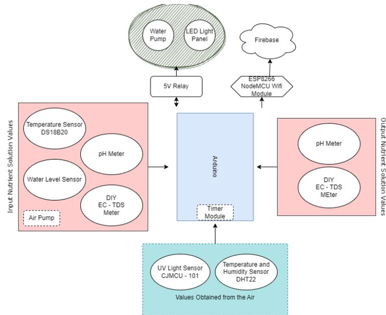
Figure 1. Prototype Arduino installation diagram and demonstration
