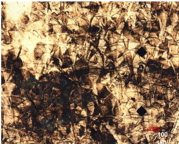
Figure 30. CSS sample; 50X magnification microscopy image of region CD as described in Figure 26
