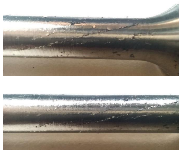
Figure 7. SSS tensile specimens with surface cracks during threading
