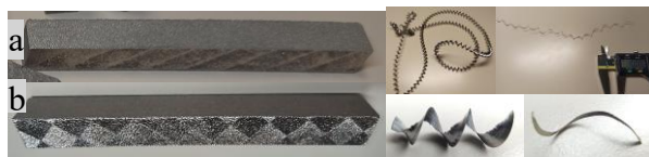
Figure 5. Square cross-section bars produced by the (a) SSS (b) CSS from which the tensile test specimens are obtained. (c) Chips formed in the manufacture of tensile test specimens
