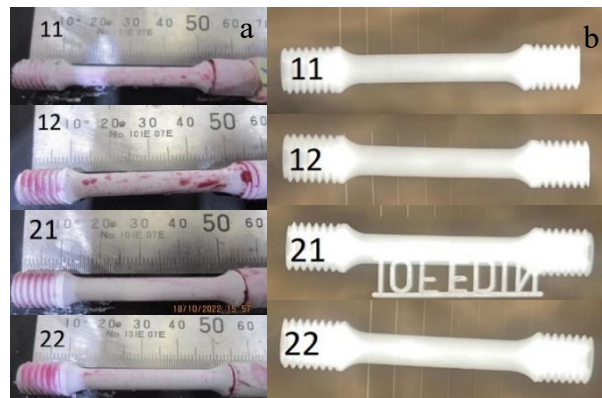
Figure 8. Penetrant test (a) and radiography result (b) photos
