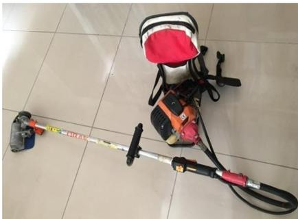
Figure 2. Brushcutter mounted log debarker (B-Debarker)
