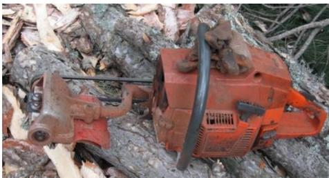
Figure 1. Chainsaw mounted log debarker (C-Debarker)
