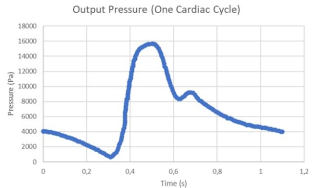
Figure 5. Outlet pressure conditions during one cardiac cycle.
