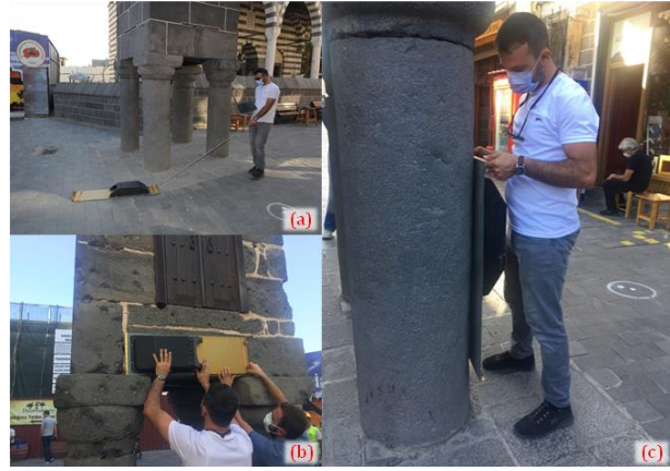
Figure 8. A typical application of the GPR on: (a) the ground of the surrounding area of the minaret, (b) the basalt lintel of the minaret, and (c) the column of the minaret
