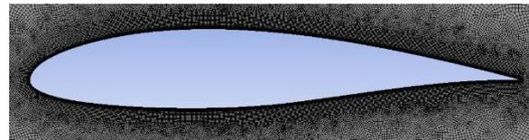
Fig. 4. Detailed mesh on the airfoil surface.
