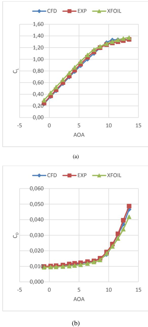
**Fig. 6.** Comparison of lift coefficient (a) and drag coefficient (b) between CFD, XFOIL and experiment at  $4 \times 10^5$  Reynolds number.
