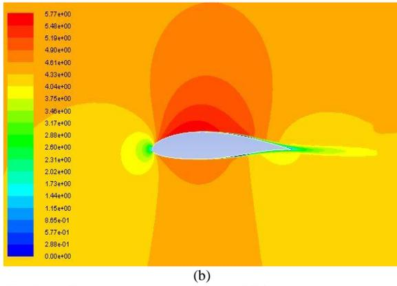
**Fig. 7.** (a) Contour of static pressure on SG6040 and (b) contour of velocity magnitude over SG6040 at 0.27 of AOA at  $3 \times 10^5$  Reynolds number.
