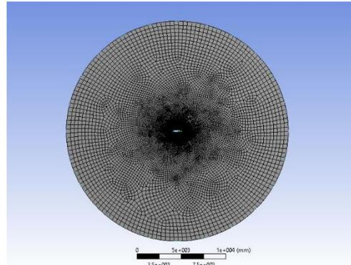
Fig. 3. The O-ring type domain structure with 25 m diameter for 2D analysis.
