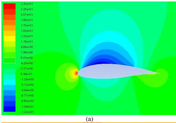
**Fig. 8.** (a) Contour of static pressure on SG6040 and (b) contour of velocity magnitude over SG6040 at 0.23 of AOA at  $4 \times 10^5$  Reynolds number.
