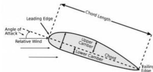
**Fig. 1.** Basic geometry of airfoil [2].
