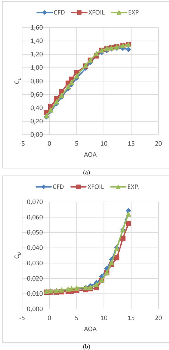
**Fig. 5.** Comparison of lift coefficient (a) and drag coefficient (b) between CFD, XFOIL and experiment at  $3 \times 10^5$  Reynolds number.
