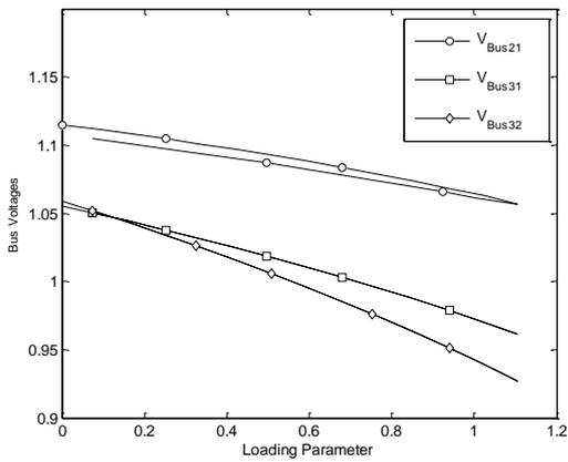
Figure 9. With TCSC 21, 31, 32 Bus Loading Parameter
