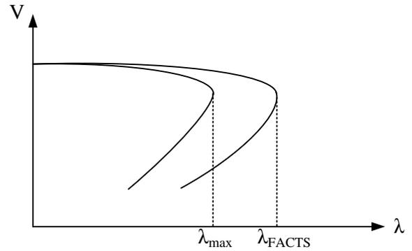
Figure 4. Relation Voltage-Maximum Loading Parameter with FACTS
