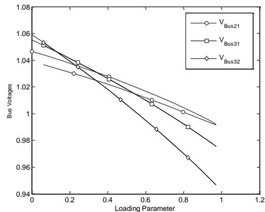
Figure 7. Without FACTS 21, 31, 32 Bus Loading Parameter
