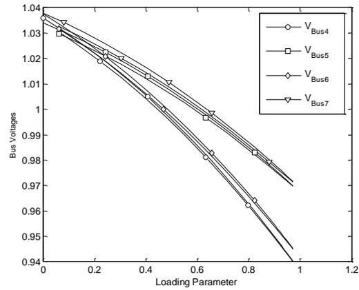
Figure 6. Without FACTS 4, 5, 6, 7 Bus Loading Parameter
