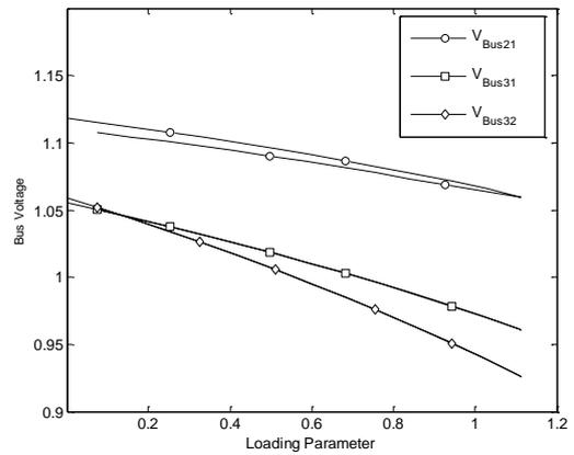
Figure 11. With SSSC 21, 31, 32 Bus Loading Parameter
