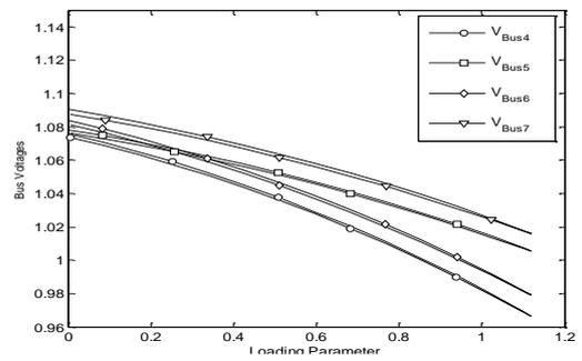
Figure 12. With UPFC 4, 5, 6, 7 Bus Loading Parameter
