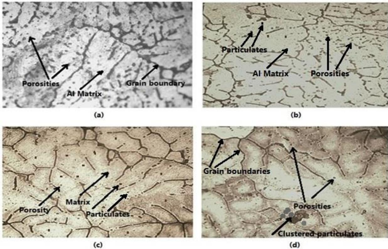
**Fig 4.** Optical micrographs of as casts (a) A356 alloy (b) 3 wt. % 115-µm desert date reinforced aluminium matrix composite (c) 12 wt. % 115-µm desert date reinforced aluminium matrix composite (d) 15 wt. % 115-µm desert date reinforced aluminium matrix composite (100X magnification)
