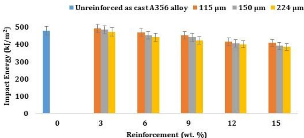
Fig 7. Impact energy of the as cast alloy and composites with varying wt. % of desert date particulates
