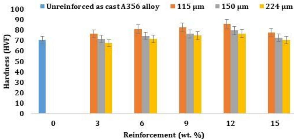
Fig 6. Hardness of the as cast alloy and composites with varying wt. % of desert date particulates
