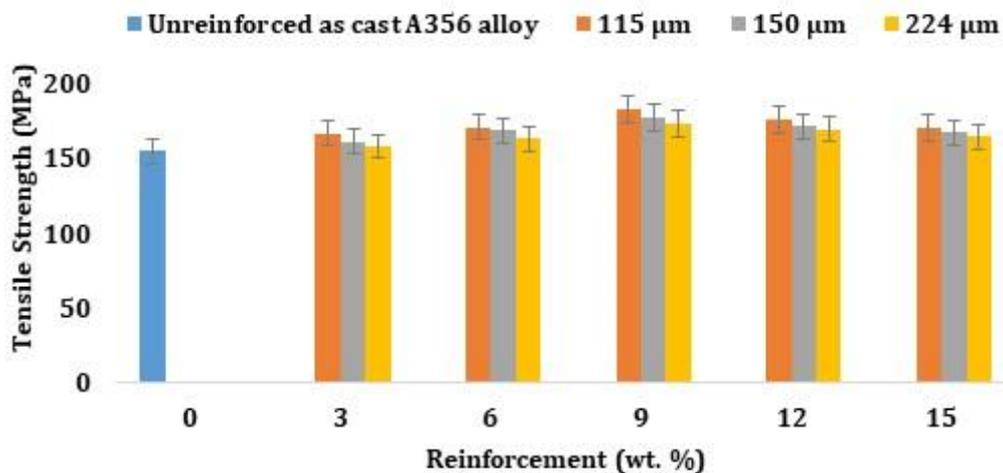
**Fig 5.** Tensile strength of the as cast alloy and composites with varying wt. % of desert date particulates
