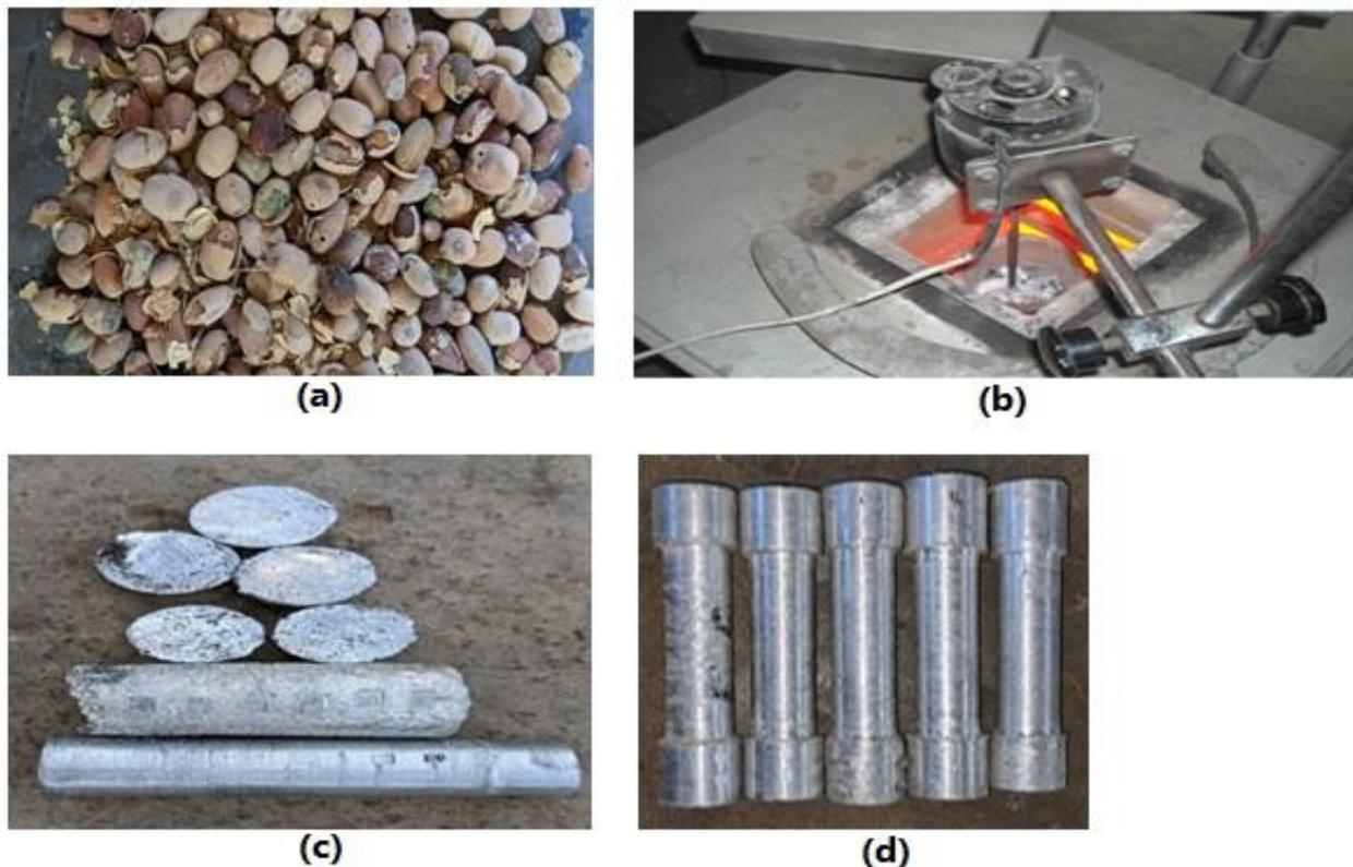
**Fig 1.** Photograph of materials and melting operation (a) Desert date fruits (b) materials melting and stirring (c) cast specimens for hardness and microstructural tests (d) tensile test specimens
