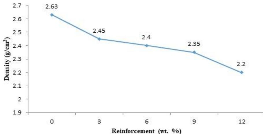
**Fig 2.** Density of the as cast alloy and composites with varying wt. % of desert date particulates
