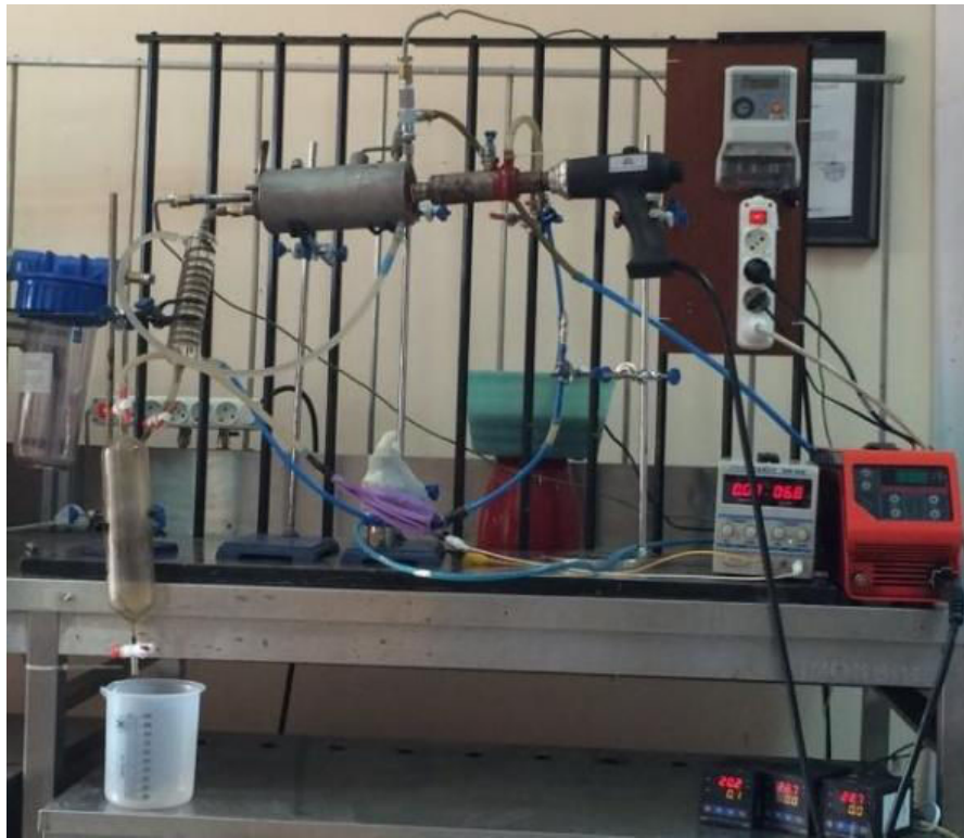
Figure 2. Plasma gasification test system.
