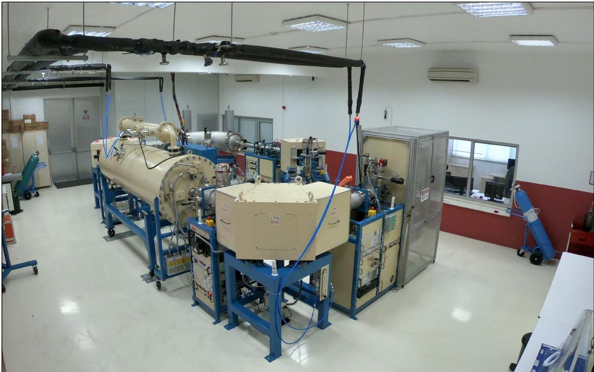
Figure 1- The AMS system in TÜBİTAK AMS laboratory room.
