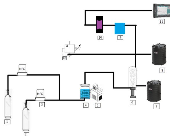
**Figure 3.** Experimental setup of CO<sub>2</sub> absorption.
