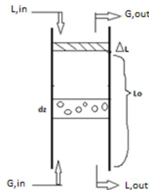
Figure 1. Schematic representation of two film theories
