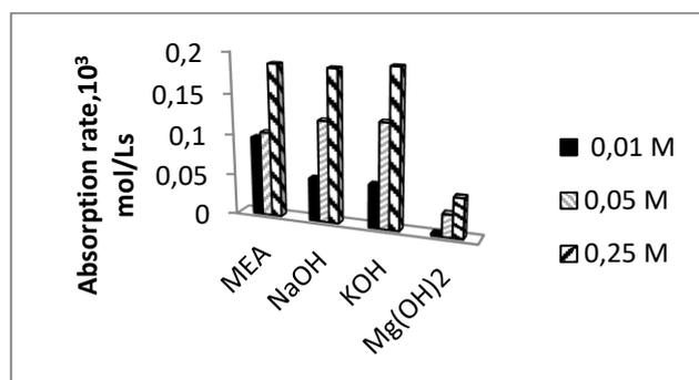
**Figure 6.** Effects of solvent concentrations on absorption rate.
