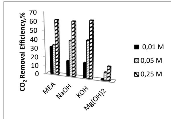
Figure 4. Effects of solvent concentrations on CO<sub>2</sub> removal efficiency.
