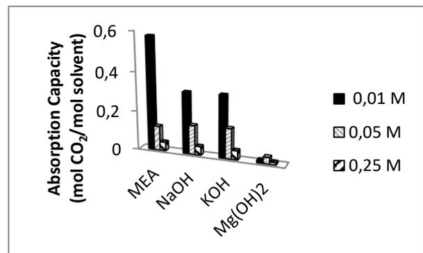
Figure 5. Effects of solvent concentrations on absorption capacity.
