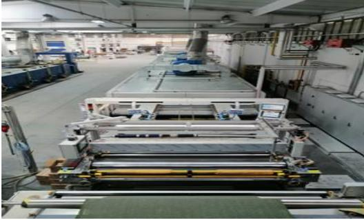
Figure 6. Stenter machine
