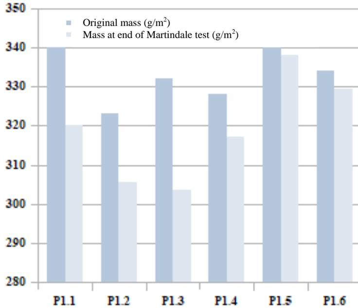
Figure 11. Mass loss for polyester samples
