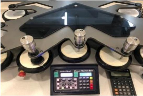
Figure 7. Martindale test device
