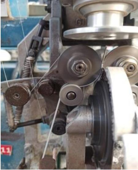
**Figure 4.** Adding fusible yarn to chenille yarn production
