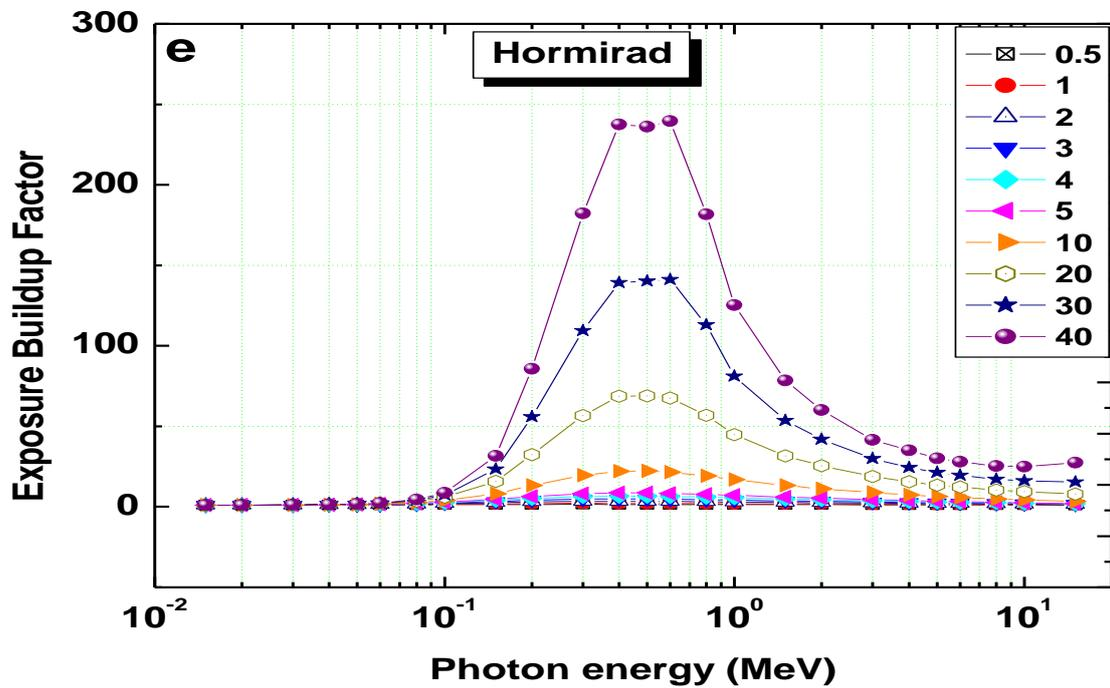
Fig.2. Exposure buildup factors of shielding materials
