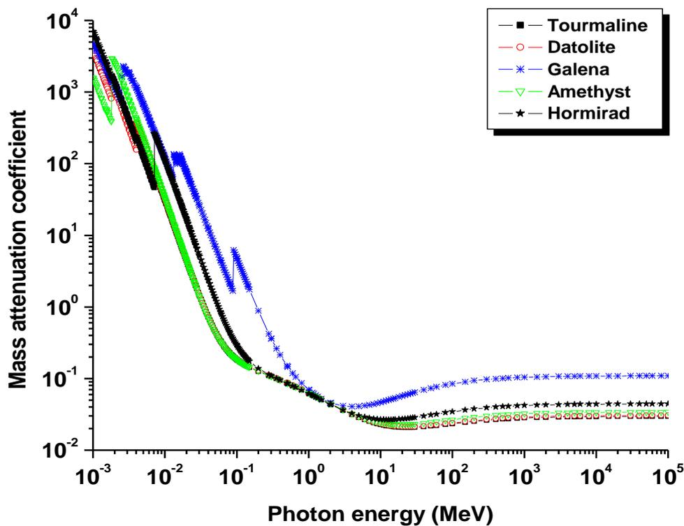
Fig.1. Mass attenuation coefficients of shielding materials
