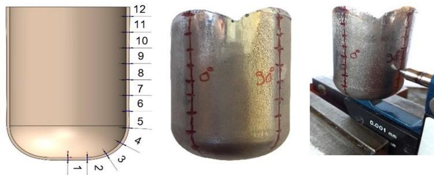
**Figure 3.** Measuring positions of the drawing cups
