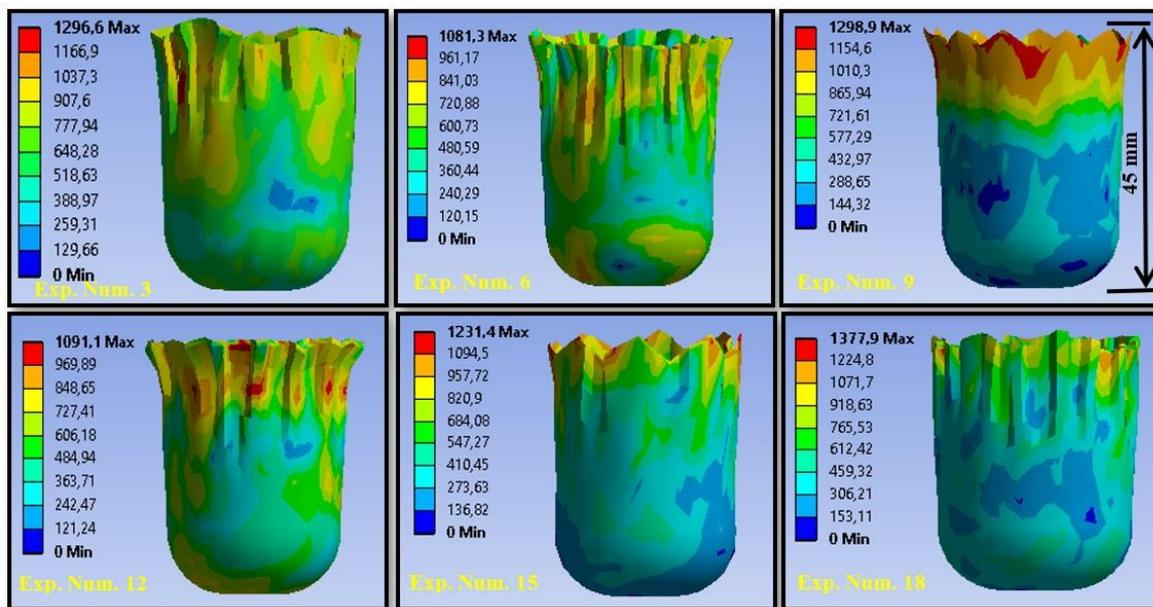
Figure 8. Stresses created by punch forces on the cup according to numerical analysis results
