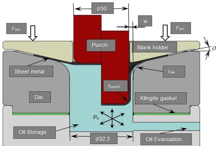
**Figure 1.** Schematic illustration of die surface angled hydromechanical deep drawing process
