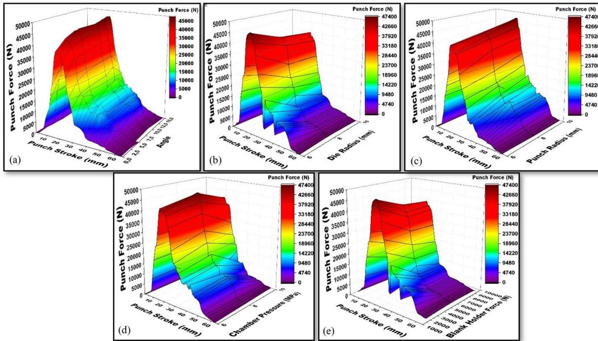
Figure 7. The effect of parameters on punch force change
