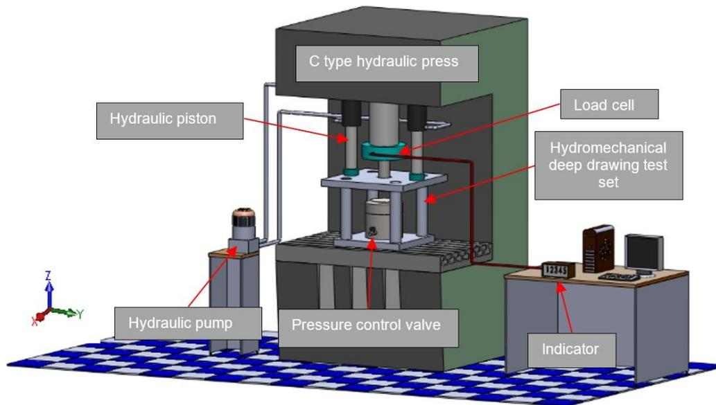
**Figure 2.** Experimental equipment of die surface angled hydromechanical deep drawing process
