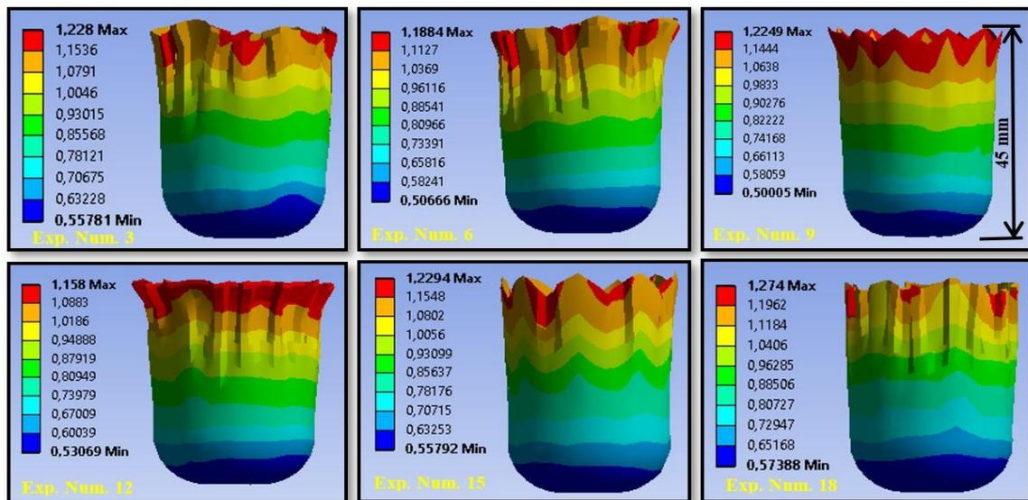
**Figure 6.** Cup wall thickness change according to numerical analysis results
