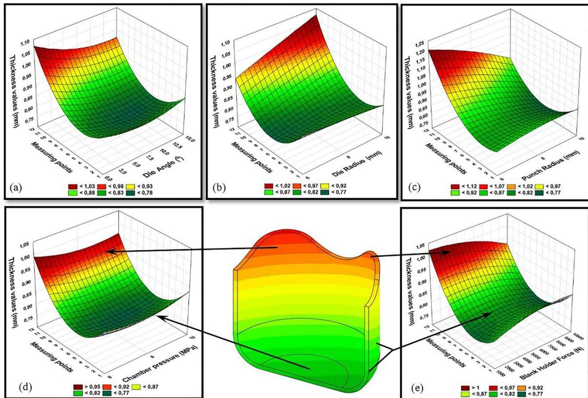
**Figure 5.** The effect of parameters on Cup wall thickness Change
