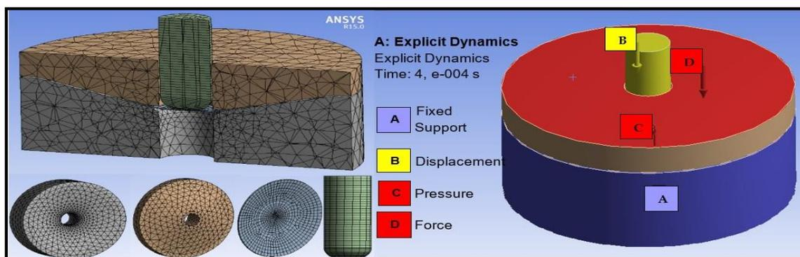
**Figure 4.** Numerical analysis mesh structure and process definitions [4]
