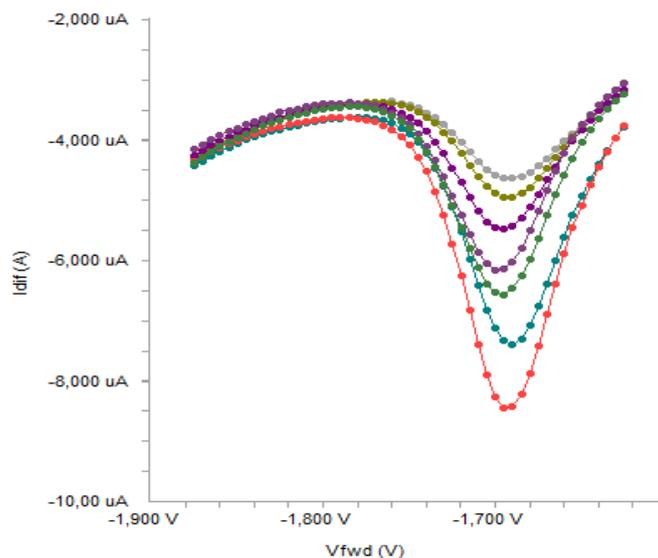
**Figure 4.** DPV voltammograms for different concentration of MX (10, 20, 40, 60, 70, 80 and 90 µg/mL) in SEs (CH<sub>3</sub>COOH\CH<sub>3</sub>COONa buffer (0.2 M, pH 4.85)/NaOH (0.2 M) (v:v, 1:1).
