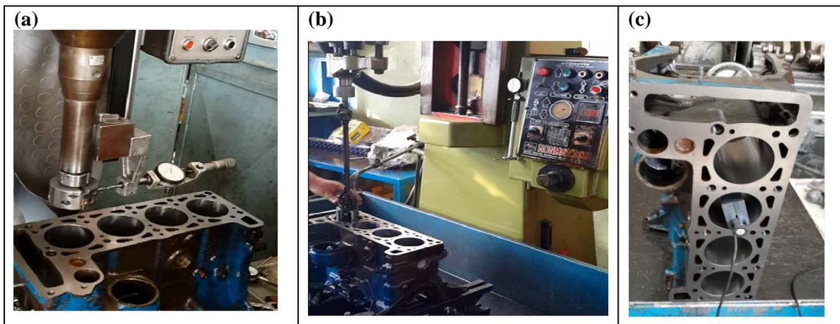
**Figure 2.** a) Rectification machine, b) Honing machine, c) Surface roughness measurement
