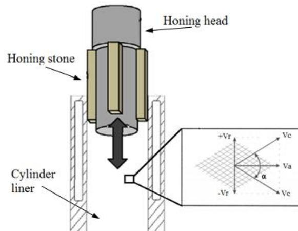
**Figure 3.** Schematic view of honing process
