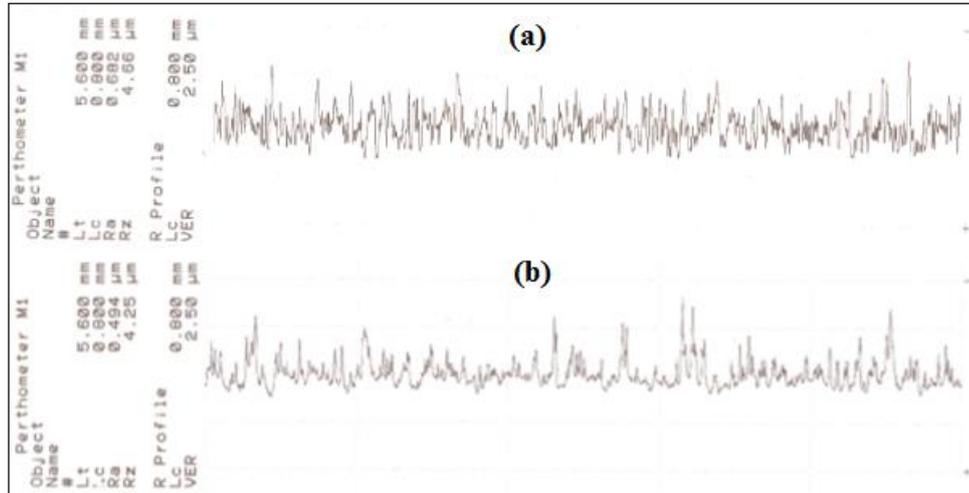
**Figure 6.** Roughness profile formed after honing; a) Rough, b) Plateau
