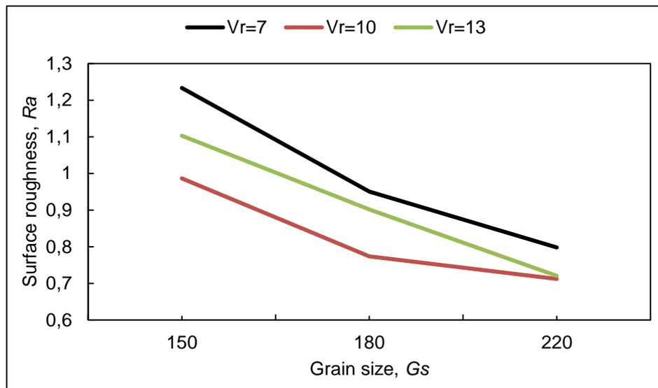
**Figure 4.** Variation of  $R_a$  versus cutting parameters
