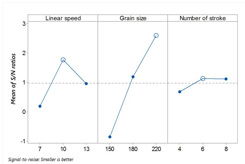
**Figure 5.** Main effect plot for  $S/N$  ratios of  $Ra$ **Table 4.** Response table of  $S/N$  ratios for  $Ra$
