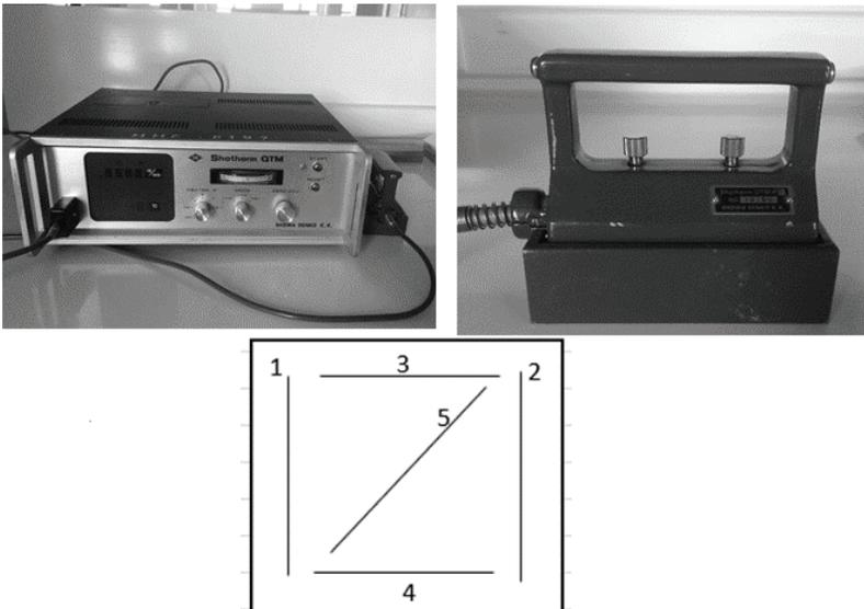
Figure 5 - Thermal conductivity equipment and measurement directions
