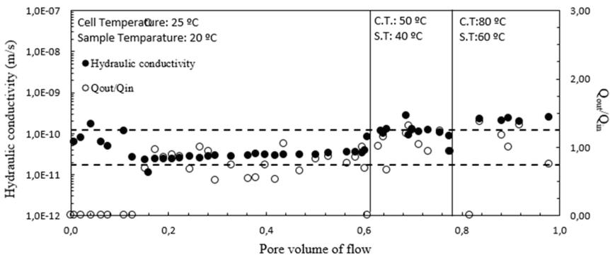
Figure 12 - Hydraulic conductivity graph in terms of pore volume of flow for 9B-81S-10PU mixture
