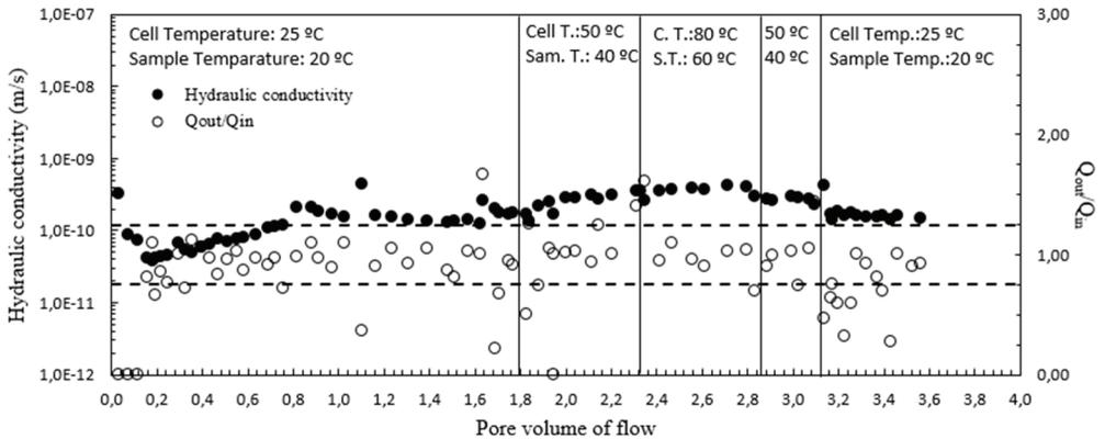
Figure 13 - Hydraulic conductivity graph in terms of pore volume of flow for 8B-72S-20PU mixture
