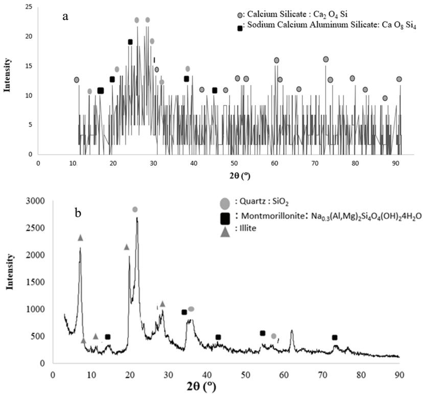
Figure 2 - The X-Ray diffraction analysis (XRD) results of the samples
