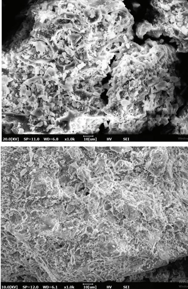
Figure 14 - Scanning electron microscope photos of the samples (x1000) (a) pumice sample at room temperature, (b) pumice sample at 80 °C
