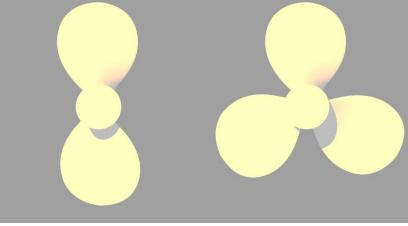
Figure 1. 3-D models of DTMB 4119
