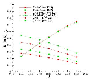
Figure 5. Hydrodynamic performance characteristics of DTMB 4119 at a constant cavitation number for different blade numbers
