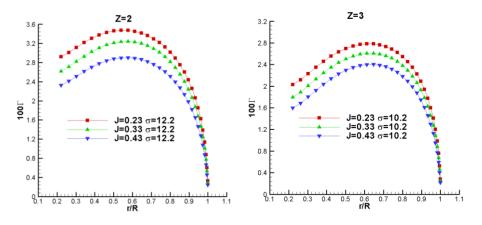
Figure 4. Circulation distribution on the blades for different blade numbers
