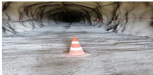
Figure 4. Conical object used in the transformation of the point cloud obtained from laser scanning.
