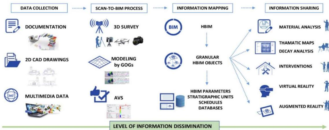
*Figure 1. HBIM process and phases of work [12].*
