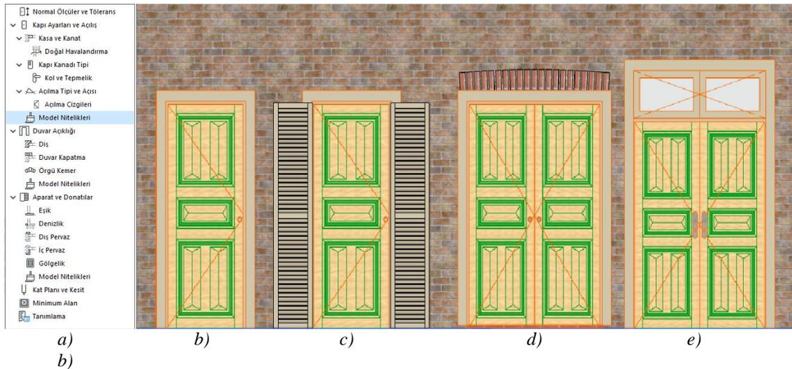
**Figure 6.** Creating door leaf alternatives as parametric objects 7a) Door parameters, 7b) single wing version 7c) Single wing, lowered version, 7d) Double-winged version with a mesh belt, 7e) Double wing, hilly version
