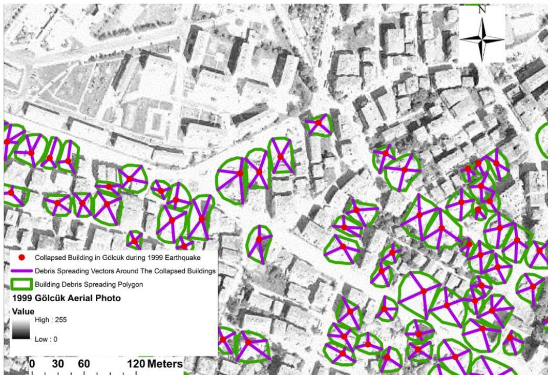
Fig 4. Building Collapse Directions in Gölçük
