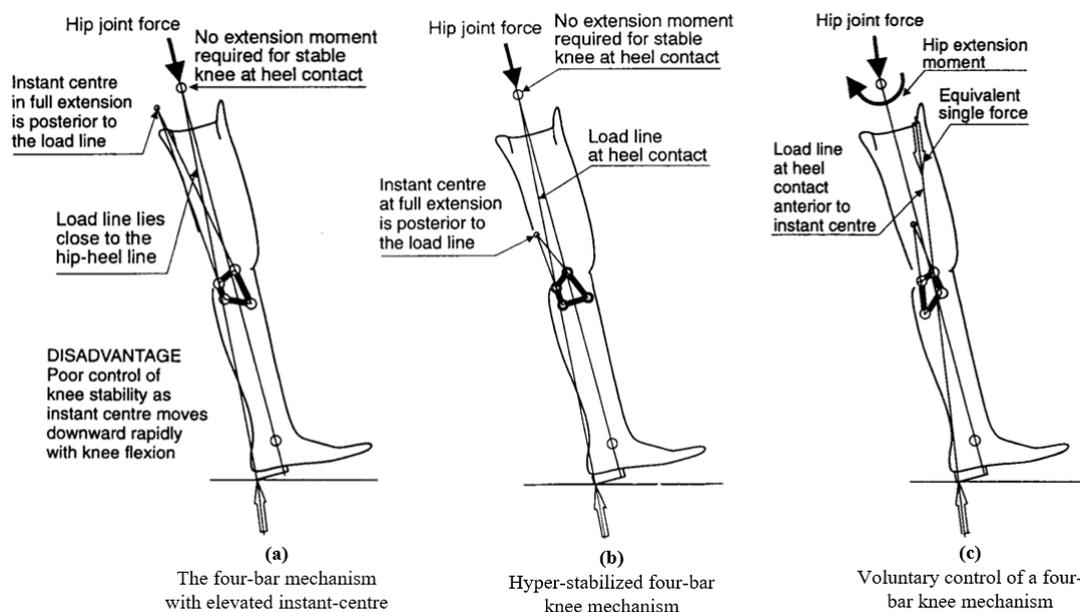
**Figure 1.** Four-bar mechanisms used in knee prosthesis (Radcliffe 1994).
