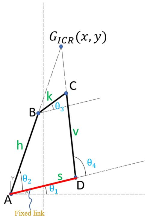
**Figure 3.** Configuration of four-bar mechanism.
