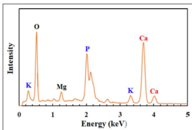
Figure 2. EDX spectra of the PLA sample.
