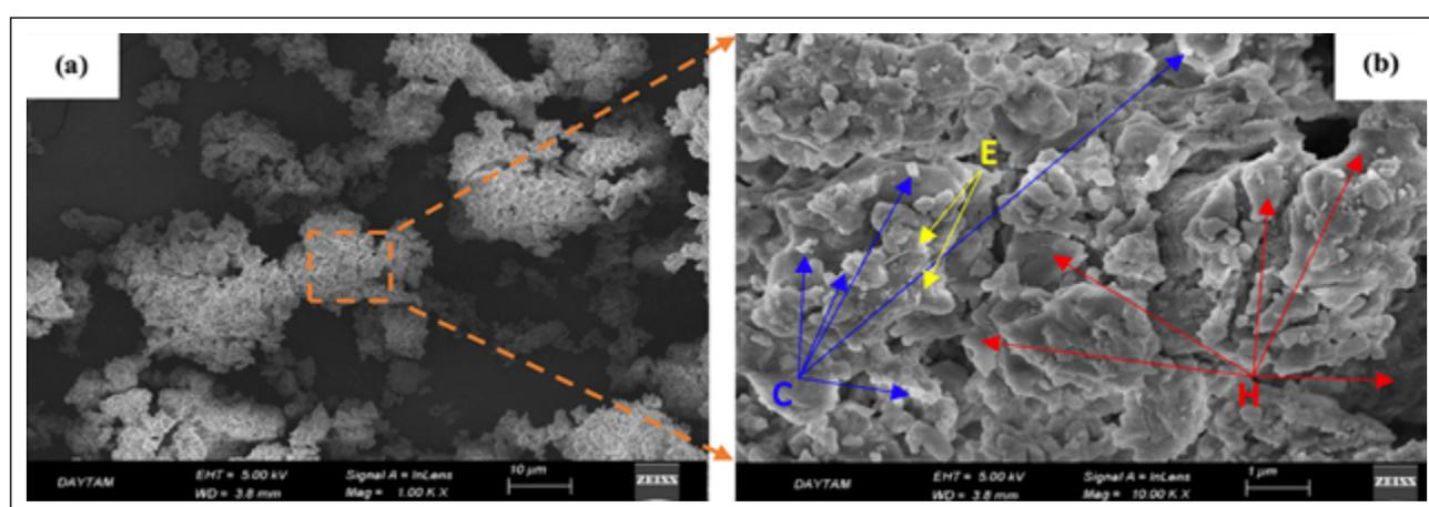
**Figure 1.** SEM images of the PLA sample. (H: Hydroxyapatite, C: Calcite and E: Ettringite).
