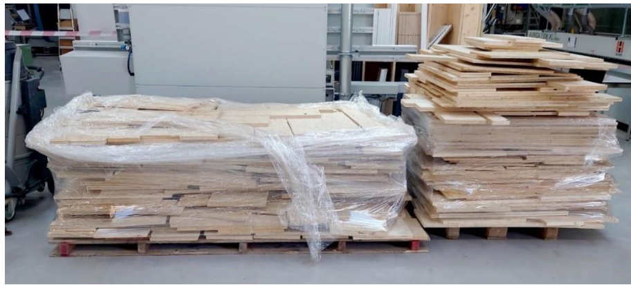
Figure 4. Material used in the project: 1.5 tons of cut-offs irregular in dimensions and properties, received from a local wood construction company, ERNE AG Holzbau
