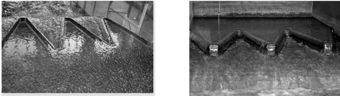
Figure 3. Experimental set-up for Trapezoidal labyrinth weirs
