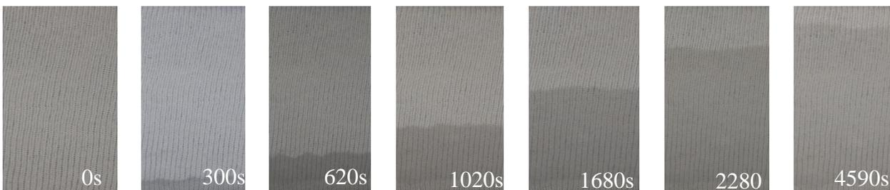
Figure 2. Wicking of distilled water into jersey-100% Cotton knitted fabric (sample 1)
