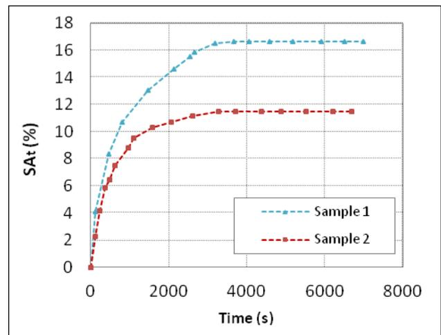
Figure 4. Experimental data of sorption ability of the Sample 1 and 2 versus time
