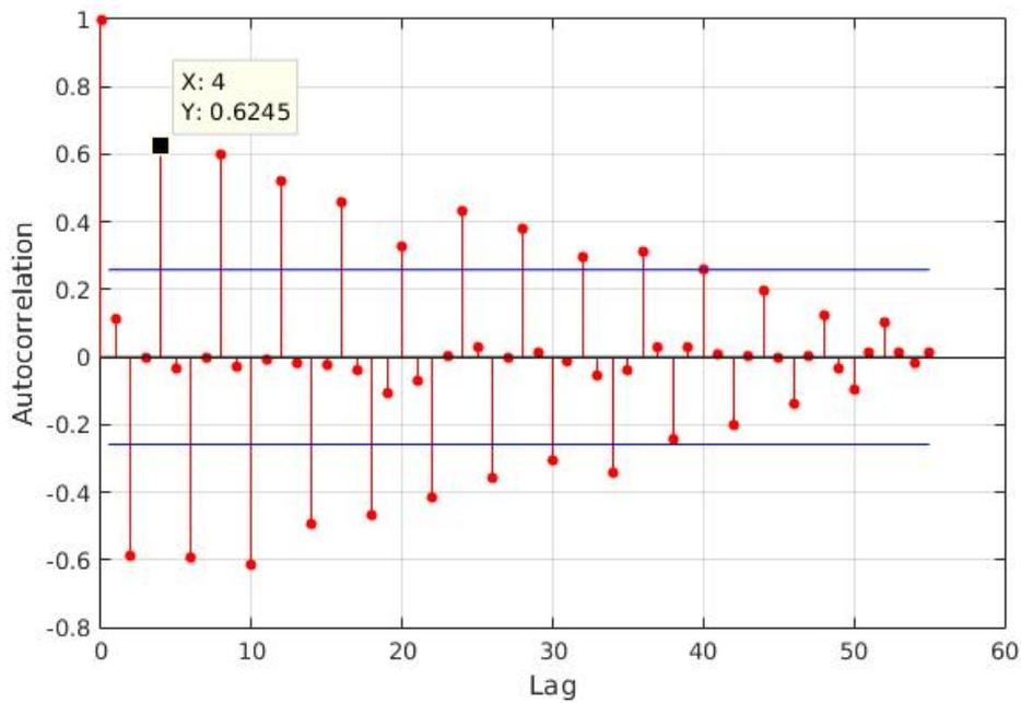
Figure 3: Correlogram of time series data of water surface by means of autocorrelation analyses.
