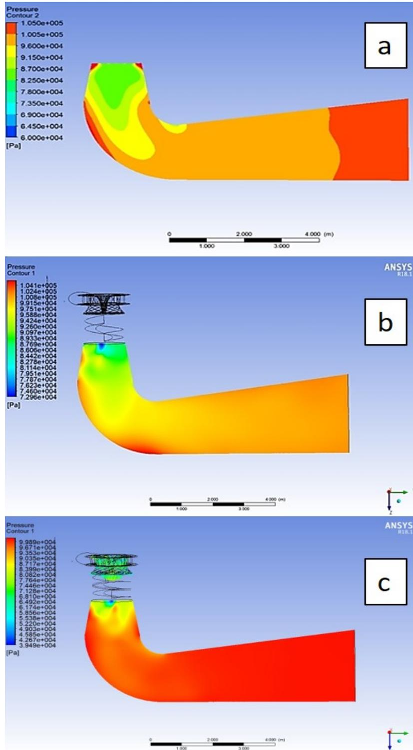
Figure 6. The pressure distributions of a draft tube for a) standard turbine, b) included one stage VPE, c) included two stage VPE.
