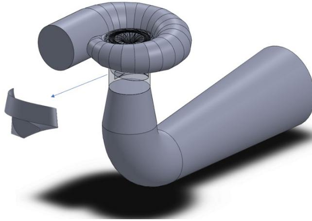
Figure 3. Numerical fluid domain of the Francis turbine having a VPE with one stage.
