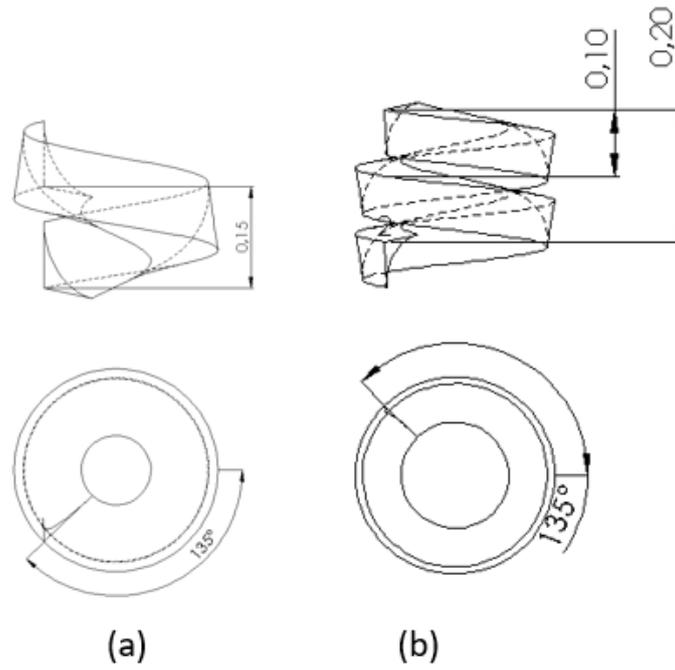
Figure 1. Dimensions of one and two staged VPE.
