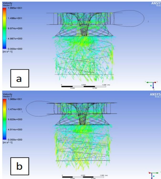
Figure 8. The velocity vectors of turbine runner for a) one stage VPE, b) two staged VPE.
