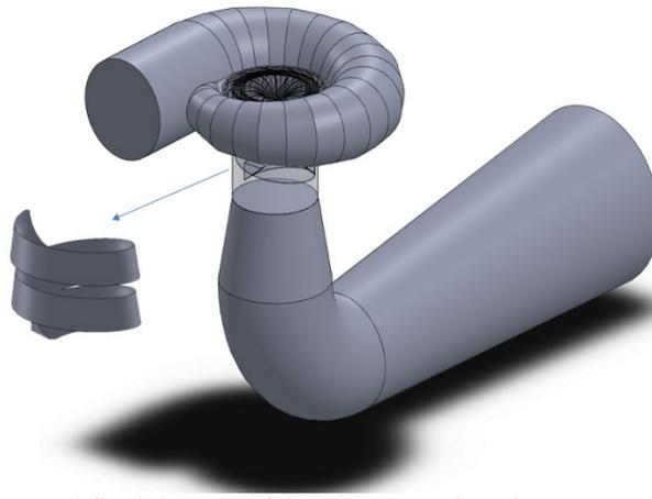
Figure 4. Numerical fluid domain of the Francis turbine having a VPE with two stages.
