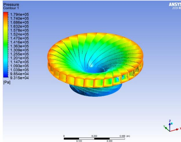
Figure 7. The pressure distribution of runner.
