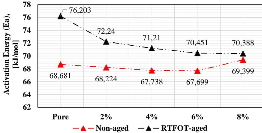
**Figure 6.** Activation energy ( $E_a$ ) values of pure and modified binders
