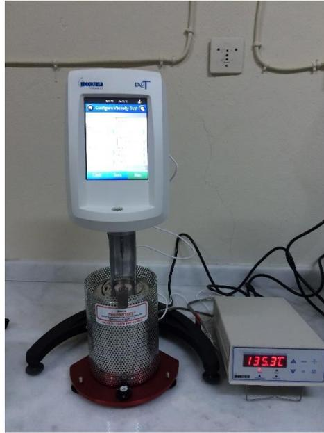
**Figure 1.** Rotational Viscometer (RV) test device
