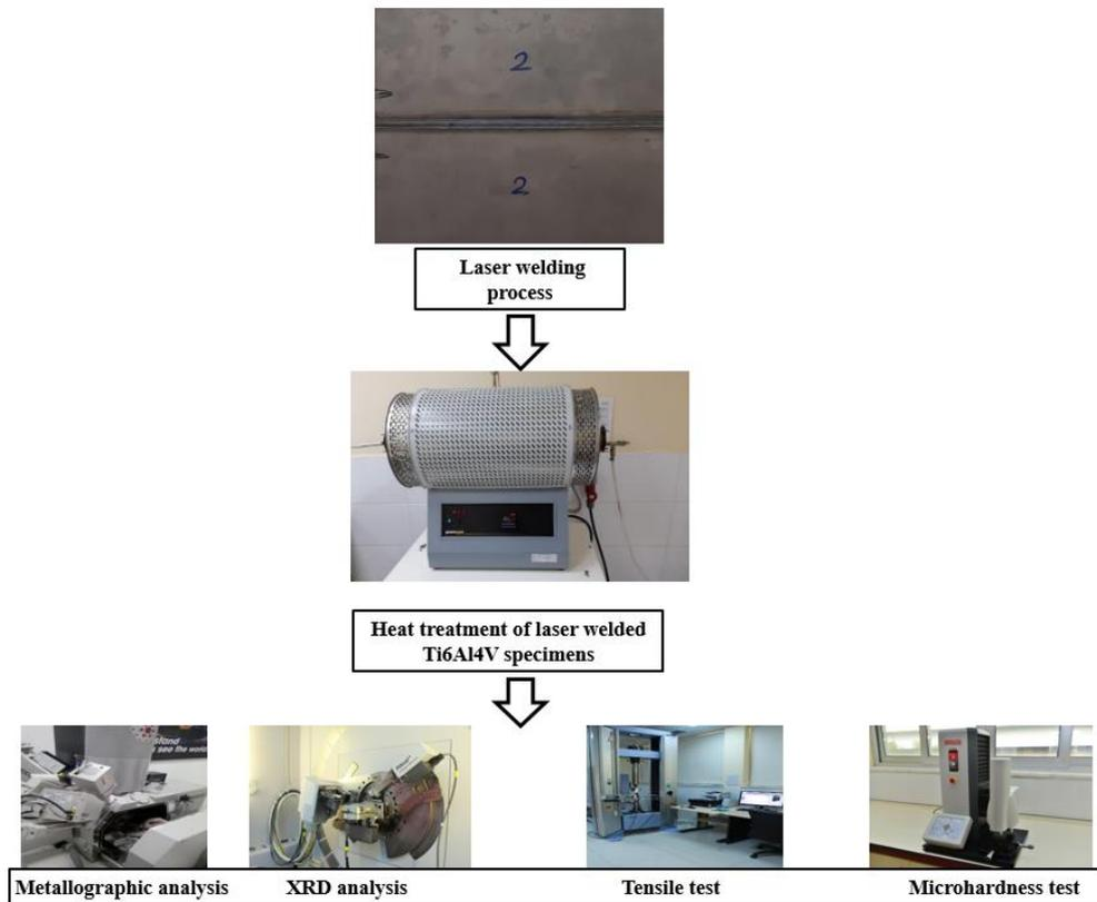
**Figure 2.** Test and analysis steps for Ti6Al4V.
