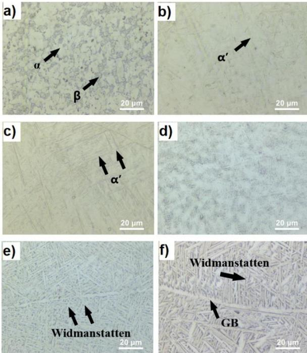
**Figure 3.** Microstructure of laser welded samples: a) base material, b) heat affected zone, c) weld zone, d) weld zone (HT1), e) weld zone (HT2), f) weld zone (HT3, GB: Grain boundary).
