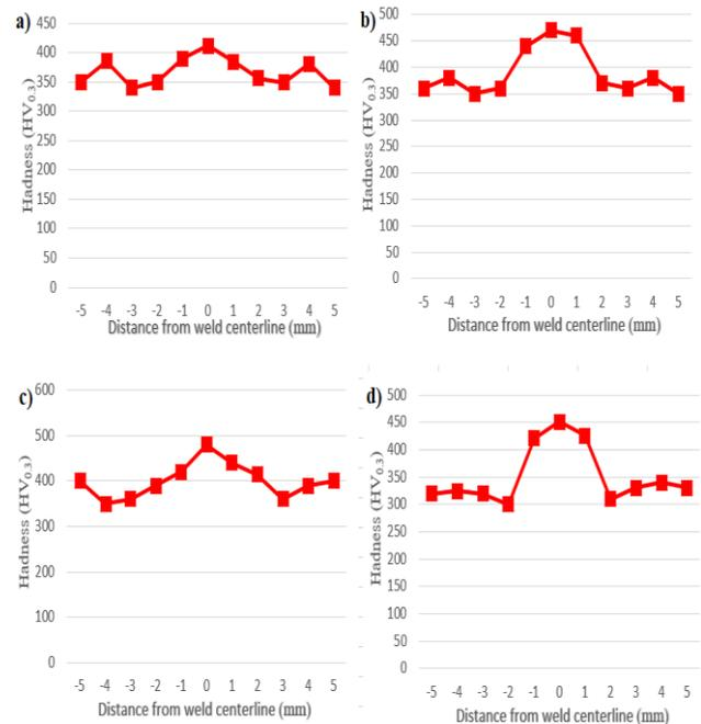
**Figure 5.** The hardness value of the samples: a) LW, b) HT1, c) HT2, d) HT3.
