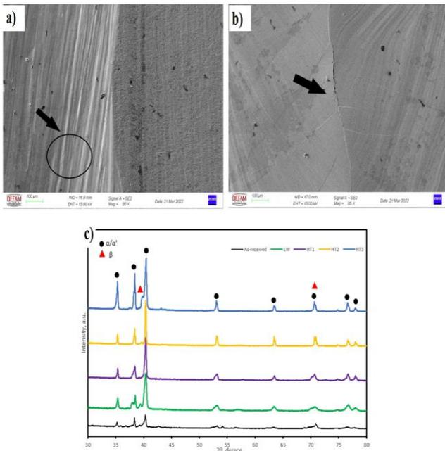
**Figure 4.** SEM view of the samples: a) General view, b) detail view, c) XRD analysis.
