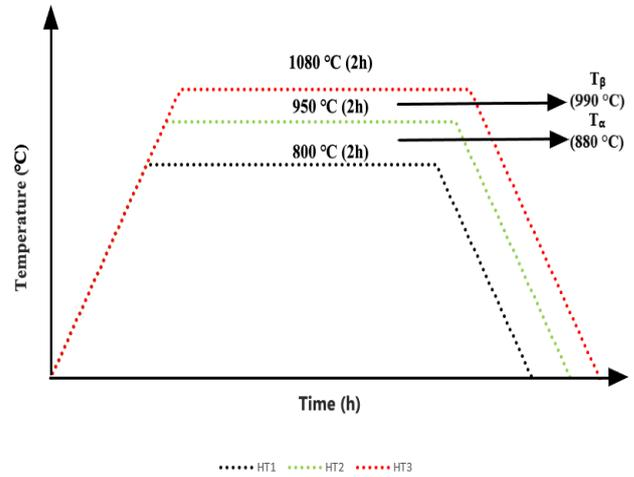
**Figure 1.** Heat treatment of laser welded Ti6Al4V materials.
