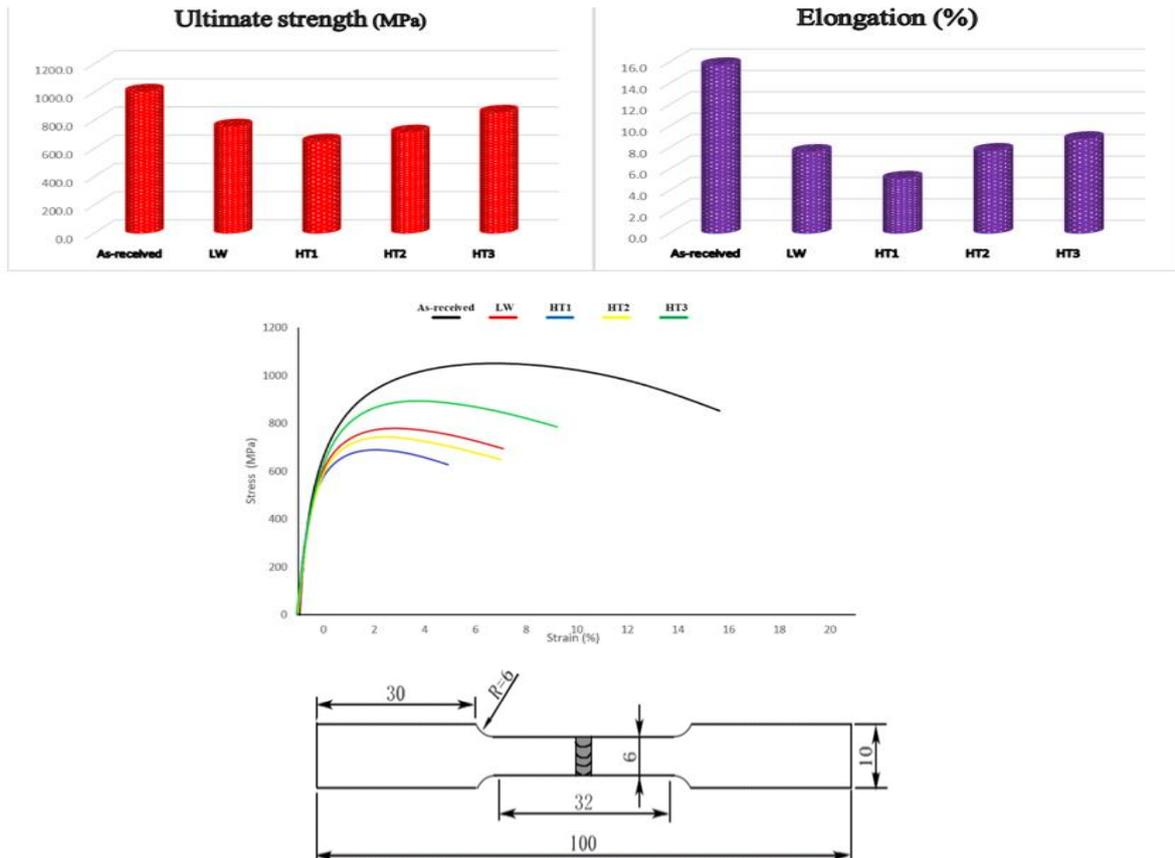
**Figure 6.** Tensile test results of parts.
