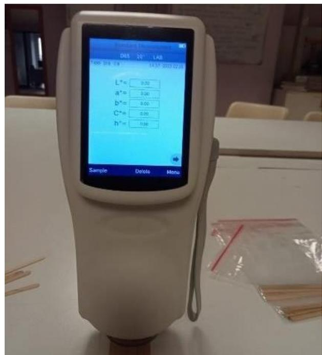
Figure 7. PCE-CSM 10 spectrophotometer device.
