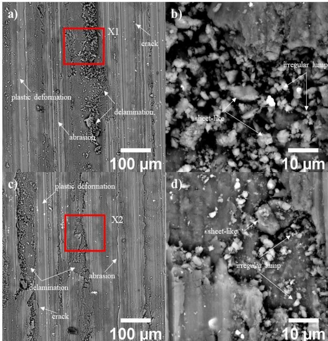
**Figure 3.** SEM images of worn surfaces under an applied load of 50 N. (a) As-cast, (b) the magnified surface (the red square part of X1 in a), (c) Solid-solution treated sample, (d) the magnified surface (the red square part of X2 in c).
