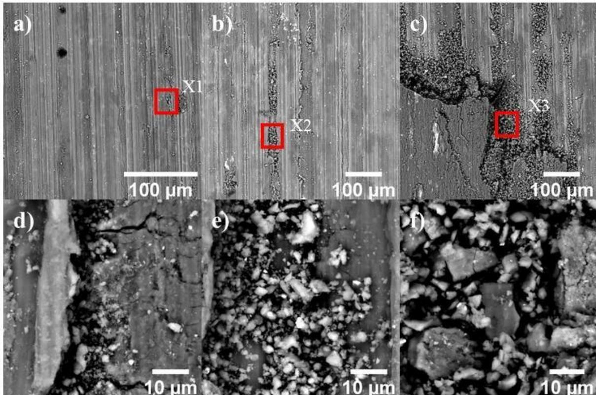
**Figure 4.** SEM images of aging treat samples at 12 hours worn surfaces under an applied load of (a) 10 N, (b) 25N and, (c) 50 N. (d-e) the magnified surface (the red square part of X1 in a, X2 in b and X3 in c, respectively).
