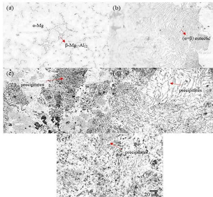
**Figure 1.** Optical images of (a) As-cast, (b) solid-solution treated, (c-e) 4-, 8- and 12-hour aged samples, respectively.
