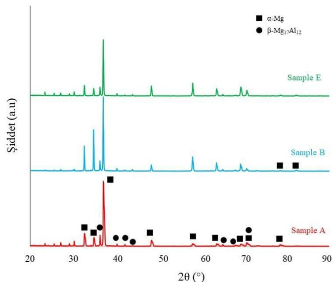
**Figure 2.** XRD analysis of selected samples indicates two crystalline phases in the crystal structure.
