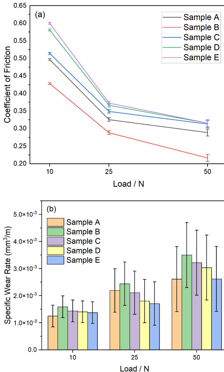
**Figure 5.** (a) Friction coefficients and (b) specific wear rates of all samples under three different (5 N, 25 N, and 50 N) applied loads.
